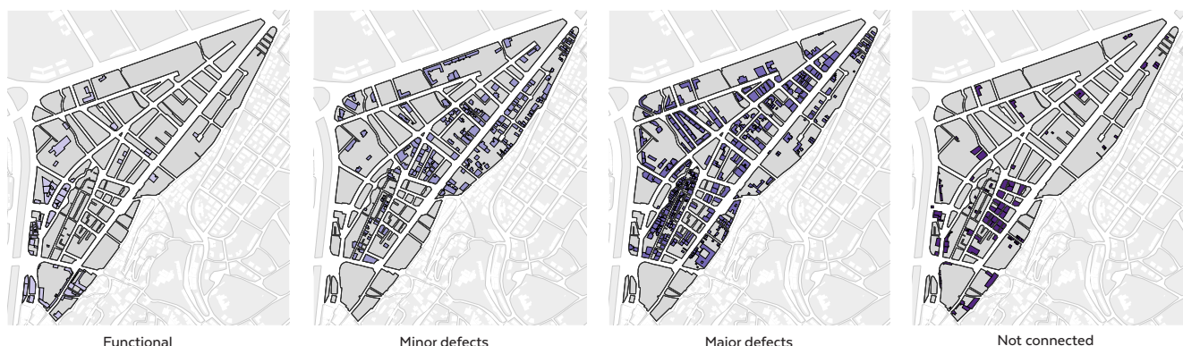
Figure 47 Condition of buildings' connection to wastewater network
