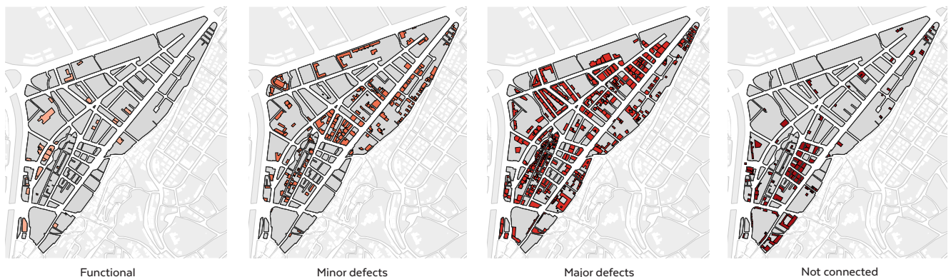
Figure 49 Condition of buildings' connection to stormwater network
