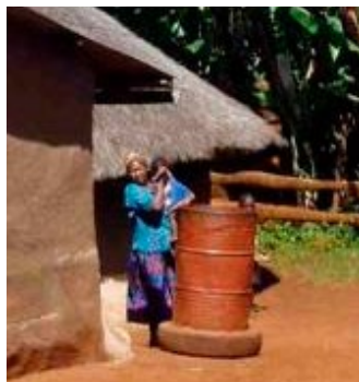
Picture 6. 10: Domestic roof water harvesting with an oil drum in Kapchorwa
