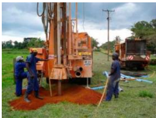
Picture 6. 6: Air percussion drilling with a big KLR rig in Luwero district
